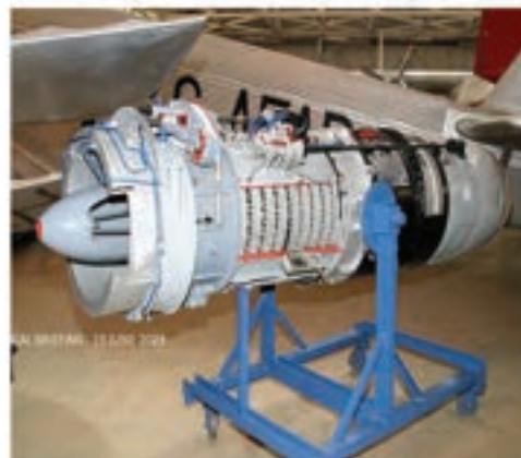
Messerschmidt 262 (Seattle Museum) and its 1942 JUMO Axial compressor Turbojet Engine.
